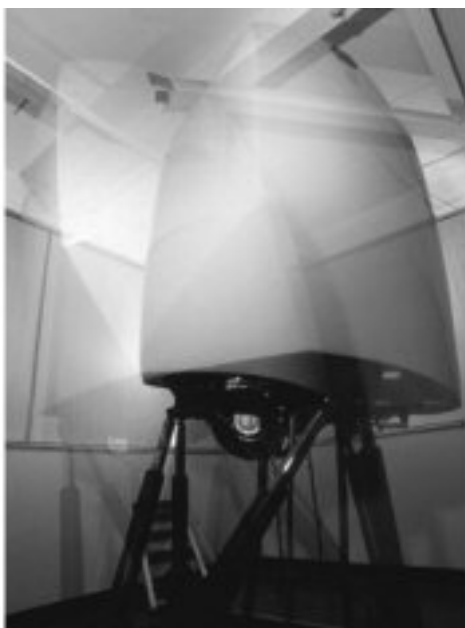
Figure 1: HELIFLIGHT 6 d.o.f. motion simulator
