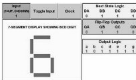
Figure 3: Simulation of BCD up/down counter with 7-segment display
