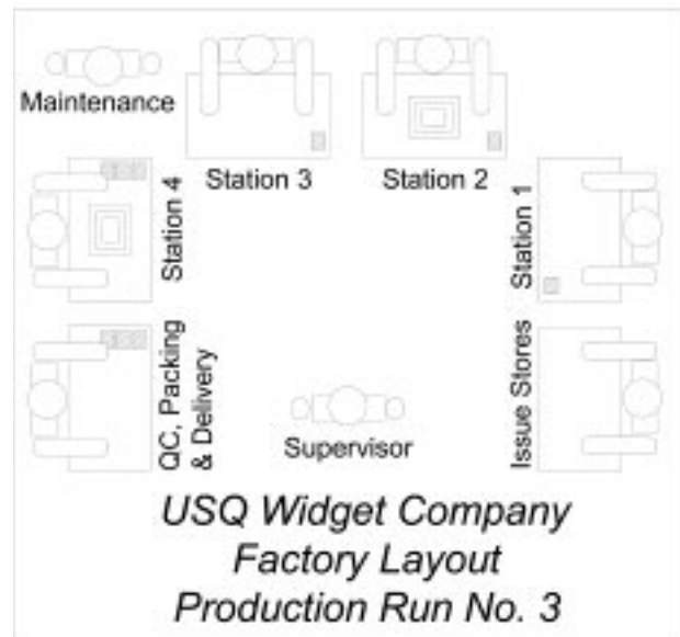
Figure 2: Layout incorporating World Class Manufacturing Techniques of efficient product flow, Just-in-time (kanban) system and elimination of 'waste'
