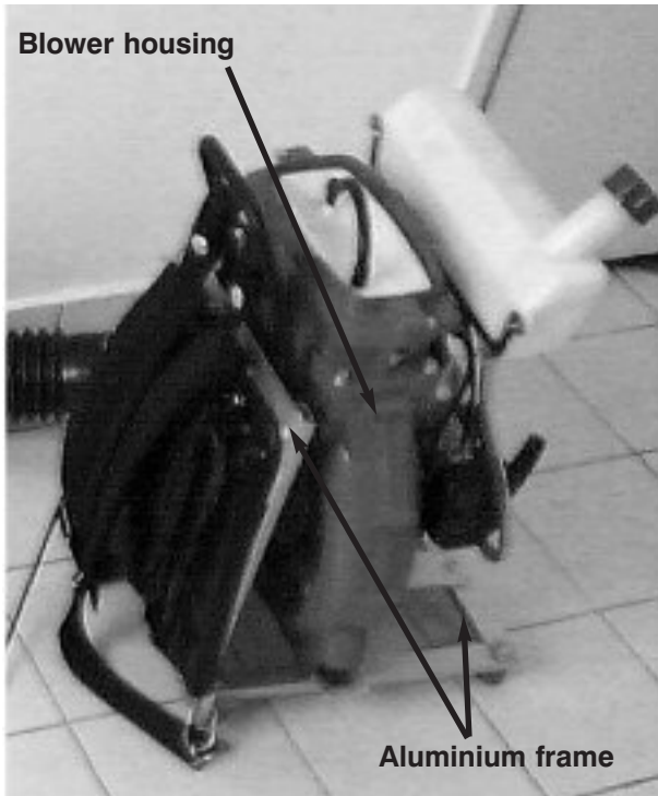
Figure 3: The prototype palm oil fruit seeds collecting machine.
