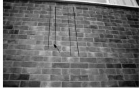
Figure 4: Accident traces of tips 'walking down wall'
